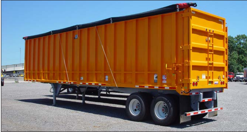
Trailer shown with optional, patented Roll-Rite electric side-to-side tarp system.
