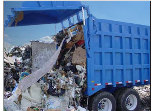
Steel push out trailers can safely unload at landfills where ground conditions are not always ideal.
