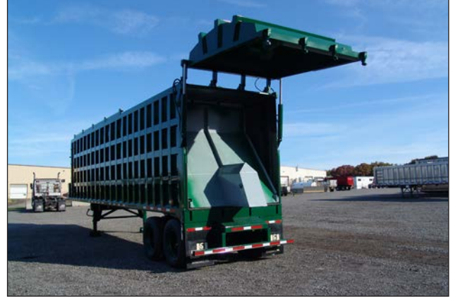
Ejector ram cylinder is sized to completely unload trailer and the replaceable UHMW wipers on top and sides of ejector ram provide superior clean-out.
